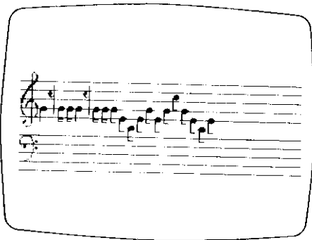
This display shows just how versatile and sophisticated the HP-85 graphics system can be. The staffs, clef marks, notes and rest marks were all drawn with the user-definable graphics operations.
