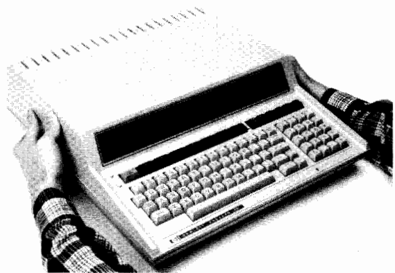
Top Cover Lifting Position
