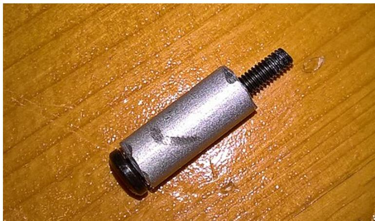
The screw also mustn't wobble inside the pipe piece and it must stick out of it for about 8 - 9 mm.
