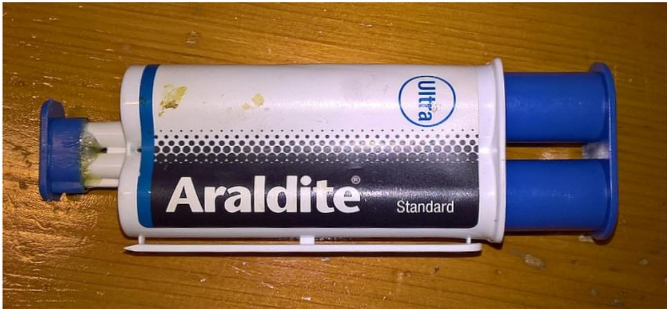
By gluing the aluminium pieces inside the standoff's holes you prevent them from doing the slightest movements, and as the standoff's plastic will be glued to the pipe with the epoxy glue it would be less likely for it to break in the future.
