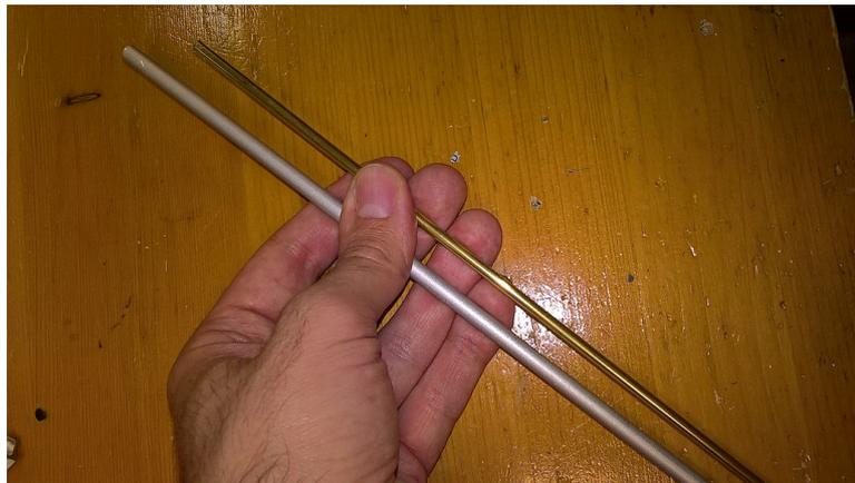
By putting the brass pipe inside the aluminium one I managed to achieve the correct centre hole diameter:
