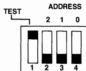
Device address switch of HP 9121D/S Disc Memory Unit.
