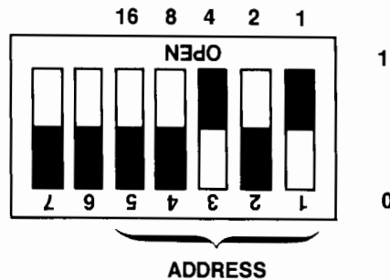
Device address switch of HP 7470A Plotter.
