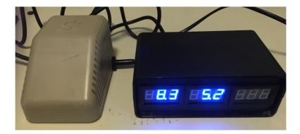
The wiring diagram is very simple: at the back there are 3 connectors bringing the measured voltages to the front instruments. A rectifier bridge is provided to measure also the alternating voltage produced by the C64 power supply, moreover some resistors allow to simulate the load, as if there were a connected device.
