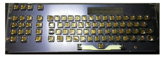
First of all, you have to clean the key from the residues of sponge in order to leave the transparent plastic disk inside the key clean enough to allow the double-sided adhesive tape to stick.
