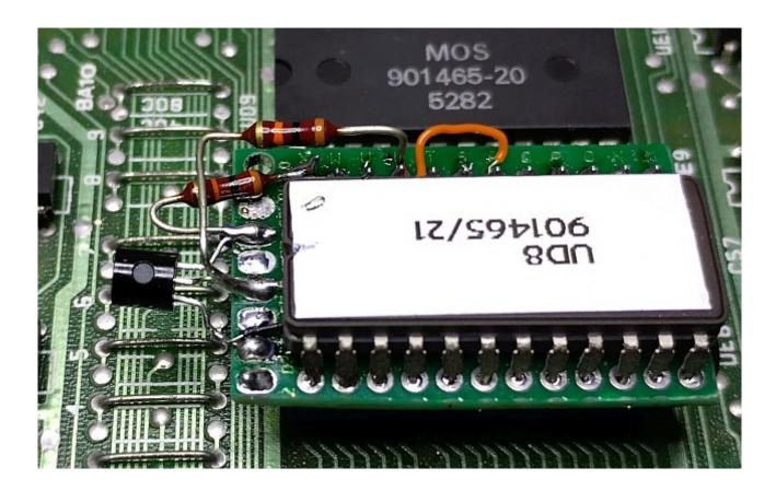
Note: on the mainboard it is present a cable which connects the 6502 CPU pin number 35 to the pin 1 of the UD3 chip (74LS393). It's not totally clear why it is connected that way, in doubt we left it there.
