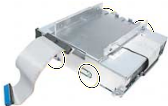
Optical Drive to Carrier Assy (4) T-10, 922-5107
